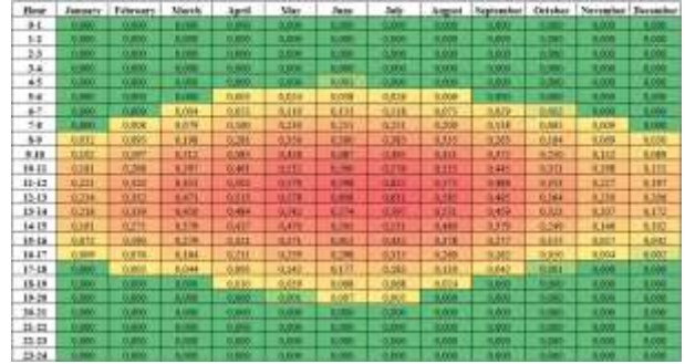
Figure 4. The monthly average hourly profile for a photovoltaic plant in Ravenna (kWh/kWp)
