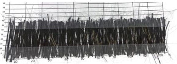
Figure 6: Fibrogram of the length distribution of rCF. y-axis: Fibre length (mm).
