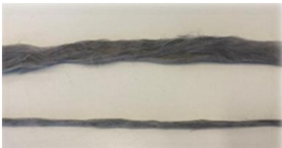
Fig. 2. Sliver (above) and roving (below) obtained through the innovative spinning process
